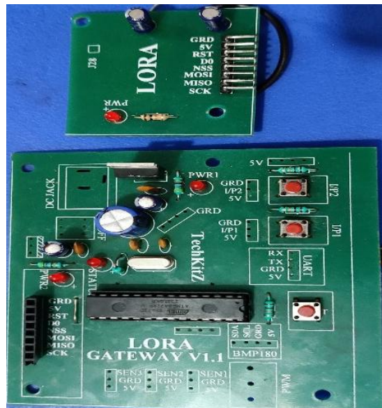
Fig .8 LoRa gateway (Transmitter and Receiver)
